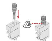
2. Insert the guide sleeve through the valve body and the coil, then screw it with a 15mm wrench;
